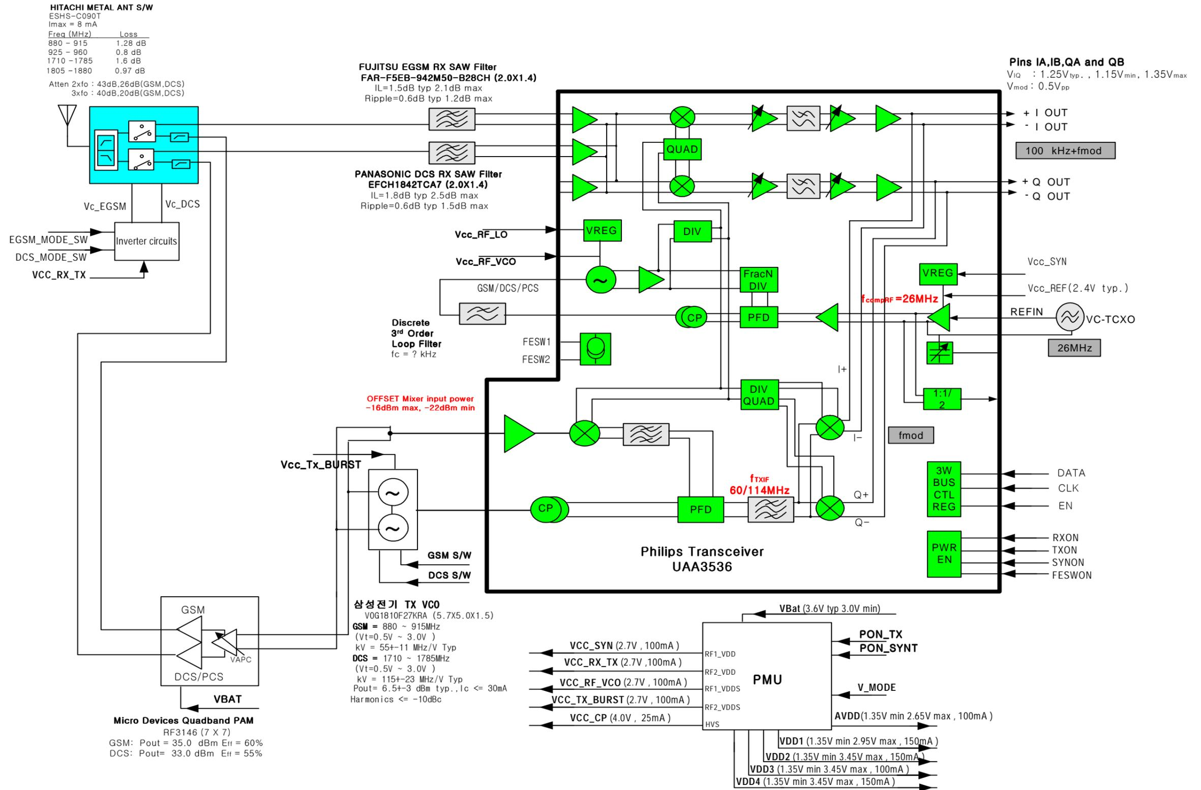
2. Base Band Solution Block Diagram
